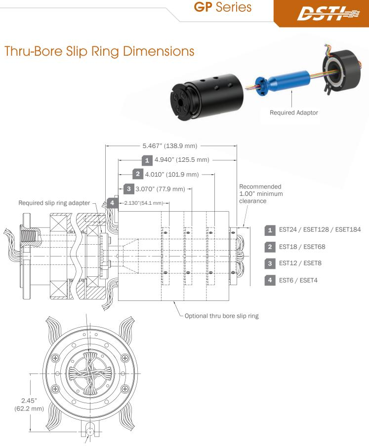
Ø.313" (7.95 mm) screw or pin for slip ring anti-rotate
