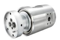
Specialized Example 1 - designed to provide hydraulic circuit for blade pitch control. Features include corrosion resistant materials for potential use in offshore environments and hydrodynamic seals with minimal oil bypass for limiting stress on the hydraulic system.
