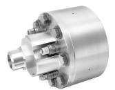
Specialized Example 2 - designed to provide rotational movement to collector piping in a parabolic trough concentrated solar power (CSP) field. Features include a high temperature packing sealing system (1,000° F), internal corrosion-resistant bearings, and a design for direct welding to the piping system.
