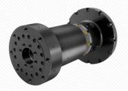
Specialized Example 2 - designed to supply grease and air service for a crusher/pulverizer application. Features include a customerspecified flange mount for integration into equipment and a design that allows for maintenance during operations with no unscheduled down time.
