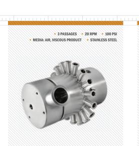
Specialized Example 1 - designed for a rotating viscous hair product filling system. Features include smooth flow passages, protected bearings for service in a wash-down environment and FDA approved seal materials.
